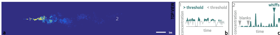
Figure 1: a) A snapshot of odor evolution in a turbulent channel. b) Only signal above a defined threshold is taken into account. c) To compute intermittency I binarize the signal, I count zero when it is below the threshold and one when above. I call "blanks" periods of time with no odor detections, while "whiffs" are periods of time of consecutive detections.
